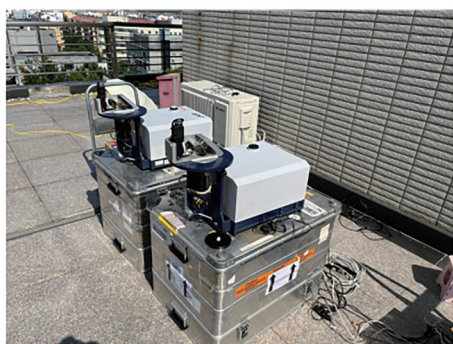
(a) 在徐州进行同时同地校准实验观测的两台 COCCON (a) Side-by-side measurements for two COCCONs in Xuzhou
